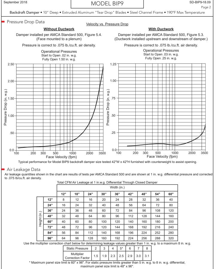
Air leakage ratings are based on AMCA Standard 500 using test set up Figure 5.4 with damper in the closed position without the aid of a counterweight or other mechanical means to provide closing torque, for a size 42"W x 42"H damper with blade and jamb seals.
